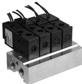
IEM Bar Manifold allows for mounting of 3-Way and 4-Way Inline valves on the same manifold. 3-Way Valves can be mounted on the same manifold to provide a Normally Closed or Normally Open function by rotating the valves 180°. 4-Way valves can be mounted with or without Flow Controls.
