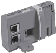
The P2M Industrial Ethernet Lite node 24DO offers 2 RJ45 ports allowing a line topology without external switch. The Ring topology can also be supported (enable/disable) for Profinet and EtherNet/IP.
