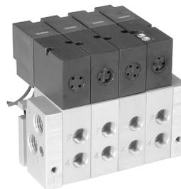
Subbase Manifold allows for mounting of 3-Way and 4-Way Subbase Valves can be mounted on the same manifold. 3-Way Valves can be mounted on the same manifold to provide a Normally Closed or Normally Open function through the use of port isolation kits. 4-Way valves can be mounted with or without Flow Controls.
