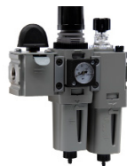
Ball Valve + Filter/Regulator + Lubricator Combinations, poly bowl 5 micron element, 116 psig (8 bar) regulator + gauge and wall mounting brackets
