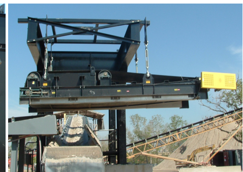
Manual Clean SPMC Shown with Side Pull Slider
