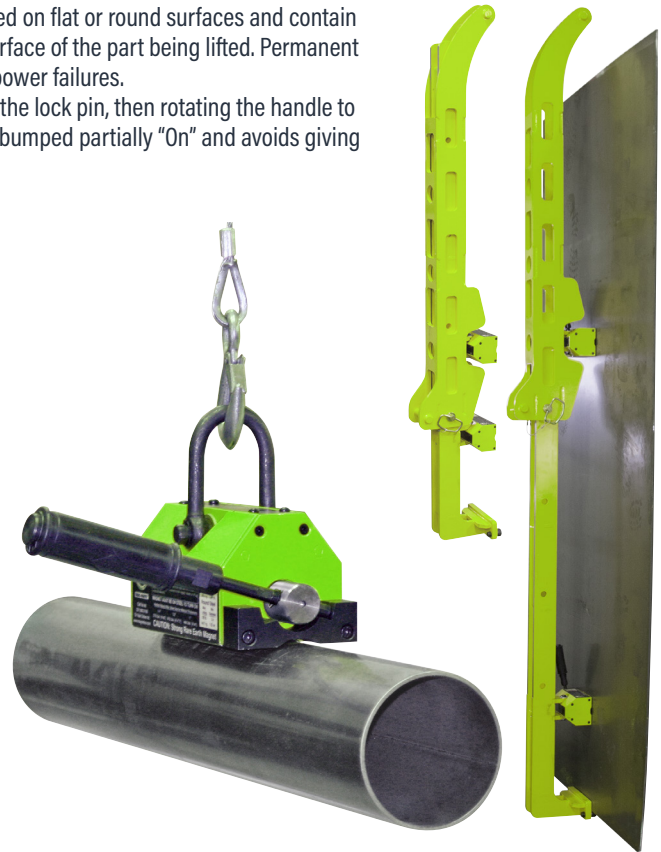
Picture above right: A customized version of IMI's Vertical Lift Adaptor featuring two PowerLift® magnets, designed to lift ferrous metal from horizontal to vertical orientation or vice versa. Adjustable for various widths, thicknesses and shapes. Ask for a PowerLift Tech Sheet for specifications.
