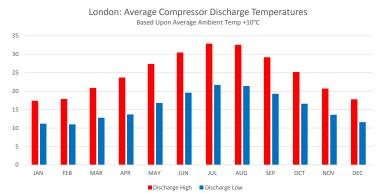
Average Max / Min compressor dischage temperatures for London were calculated based upon recorded weather data plus 10°C for after cooler discharge temperature.
