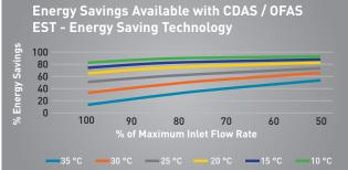
Example based upon a CDAS HL 075 / 0FAS HL 075 Purification System and referenced to a 3 Minute Standard Cycle. Energy savings are applicable to all CDAS / 0FAS models.
