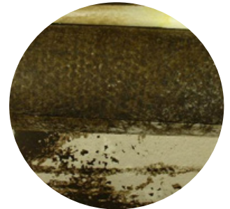
Blocked Filter Media
